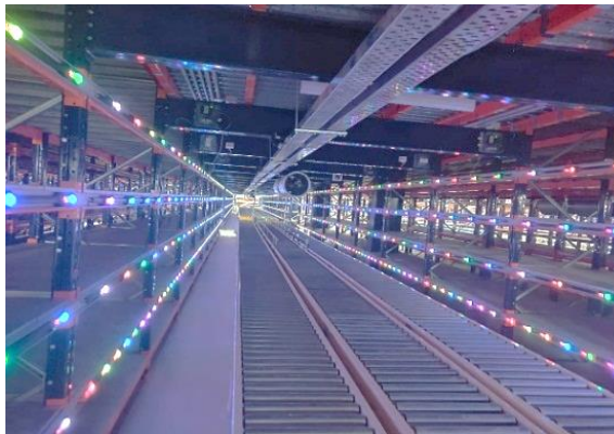
Fig.1. Warehouse using Pick-to-Light and Put-to-Light systems [4].
