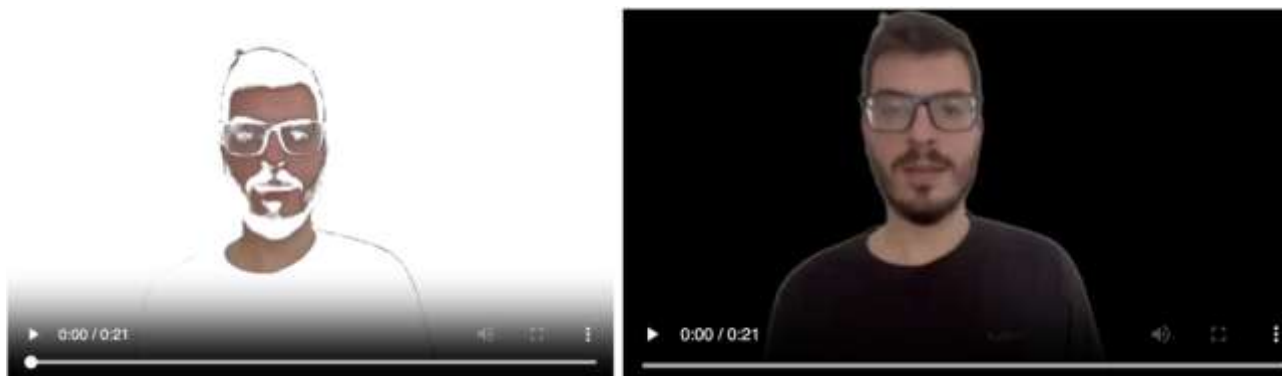
Figure 3.4: On the left is a frame of the input video in WebM format with an alpha component, while on the right is the output WebM video, which is also in WebM format, but without the alpha component.
